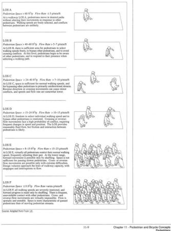
Figure 2: Visualization for highways and pedestrian walkway levels of service (Transportation Research Board 2000, 2010)
