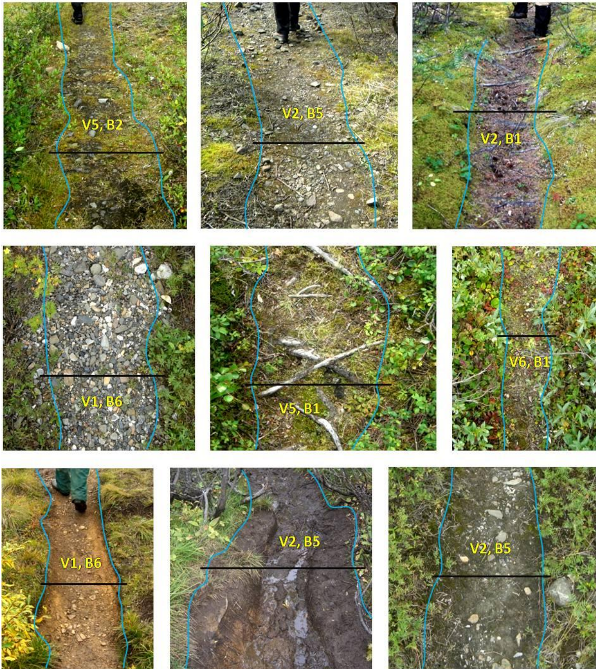
Figure 2. Representative photos illustrating the placement of telescopic antenna or shock-corded tent pole extending beyond trail borders and from which is measured veg/soil maximum incision to deepest spot along the tread. Trail width is assessed along the antenna between the blue lines. Vegetation and bare soil (see definitions and cover categories above) are assessed for the trail in a band 1 ft wide centered on the pointer. See reference assessments included in yellow on the photos. Off-site vegetation and bare soil values are assessed in representative undisturbed areas several feet beyond the ends of the pointer.
