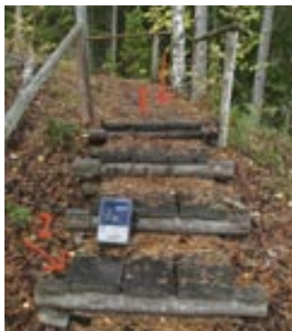
Stairs are good places to install pressure mat counters. Number 1 indicates where the pressure mat is buried and number 2 indicates where the counter is normally hidden (under the stair). RMK North-Estonian recreational area, Estonia. (PHOTO: JAAK NELJANDIK)
