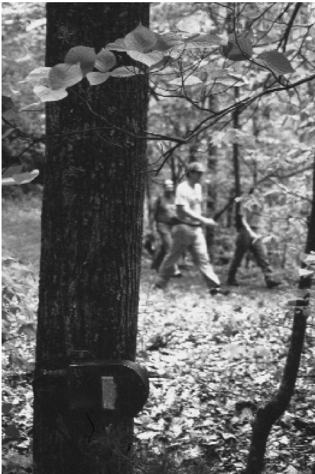
Photo-electric counters emit an infrared beam, and a reflector returns the beam to the scanner. Careful site selection and proper installation of photo-electric counters are critical to ensure accurate counts.
