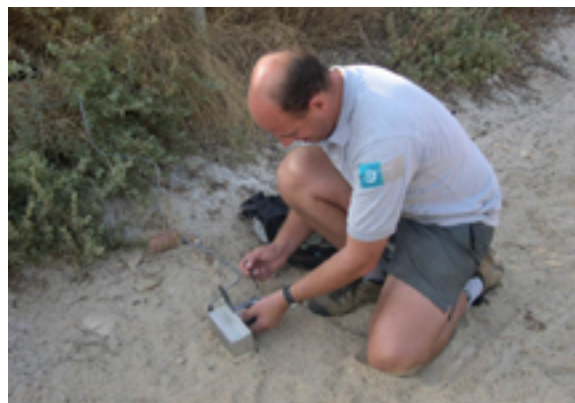
Manual read of an eco-counter on Porquerolles Island (Port-Cros National Park, France). © Credit: LETG Brest-Géomer
